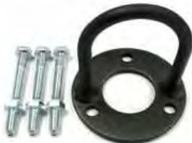
Bearing Carrier Retainer Wrench Removes and installs bearing carrier retainer nuts on MC-1/R/MR/Alpha One/Gen II, Bravo I, TRS drive units & assorted V6 Outboards Part No: 90190
